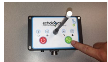
STEP 3: SELECT PIPE MATERIAL ON TRANSMITTERS.
